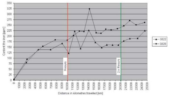
Fig. 1. The change of iron content in oil samples according to the distance in kilometers traveled a bus
