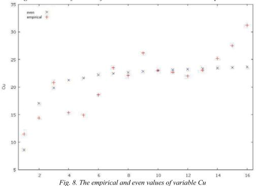
The model for the 3822 bus (the content of Fe particles)The model of type (2) seems to be the best one.Parametres:a = -283333p-value:0.001970.00001Determination coefficient: $R^2 = 0.507$ Random change coefficient:16%
