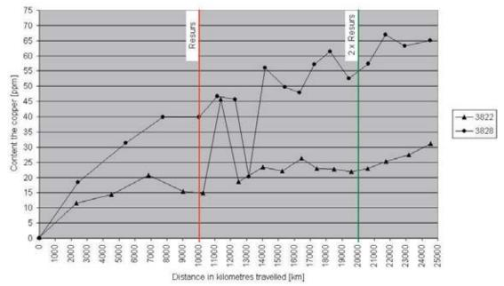
Fig. 2. The change of copper content in oil samples according to the distance in kilometers traveled a bus
